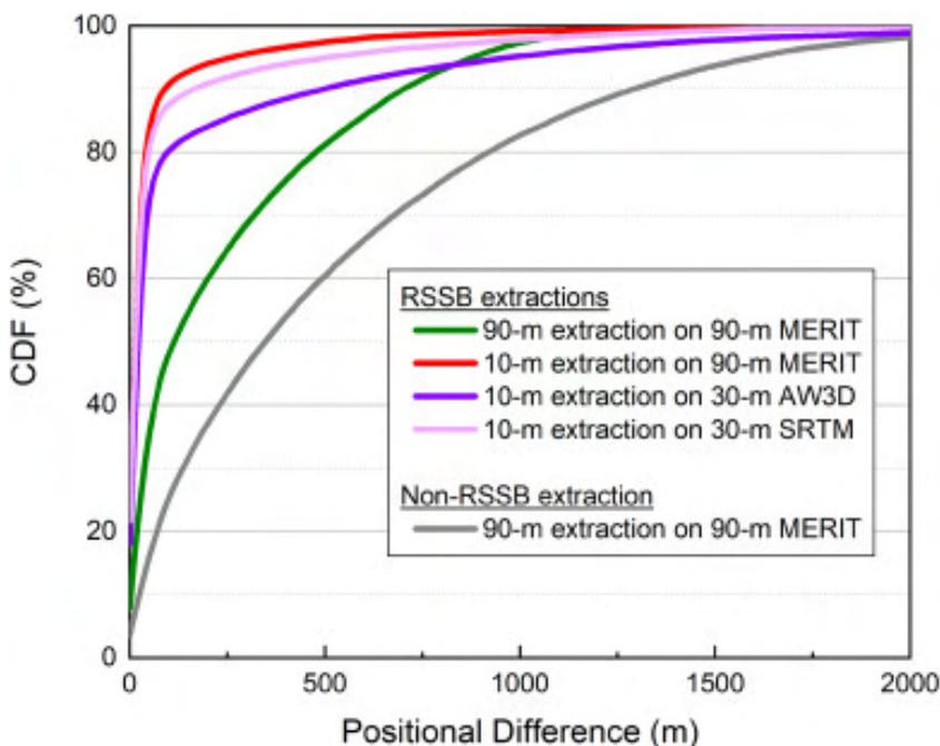
Figure 1: Location errors of river networks generated by RSSB method and conventional method (non-RSSB). The closer CDF curve near top left, the better.
