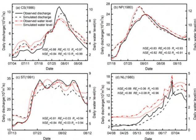
Figure 2: Observed and simulated discharge and water level hydrographs for the selected flood events
